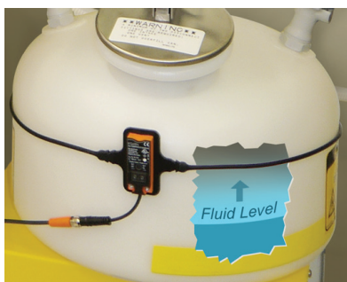
Another sensor can be set to detect high fluid level in your waste container.
